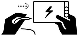
Plug the power adapter in and charge the battery (the red indicator on the left-hand side of ALBUM blinks). It is possible to switch ALBUM on and use it while charging.
